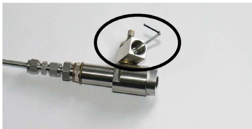
Figure 19 Removing the Leak Screw
