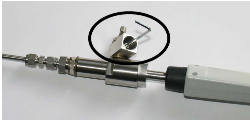
Figure 30 Removing the Leak Screw
