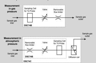
The DSC74B sampling cell enables the measurement of the sampled gas either in gas pressure up to 10 bar or in atmospheric pressure depending on the gas inlet and outlet. The DSC74C is like the DSC74B but with an additional coil to avoid back diffusion, the effect of surrounding moisture, in dew point measurements in atmospheric pressure.
