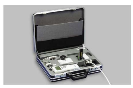
The DSS70A provides a compact solution for field checking dew point where direct measurement is difficult. Typical applications for the sampling system are metal treatment and plastics drying processes.
